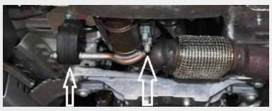
Loosen the 2 bolts that connect the down pipe to the cat back portion of the exhaust. Remove the rubber exhaust mount from the chassis. This mount will be reused to install the BBK High Flow down-pipe.
