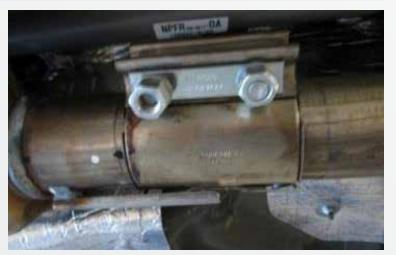
Separate the stock down-pipe from the cat back portion of the exhaust by pushing the down pipe forward towards the front of the vehicle. The down pipe comes out towards the rear of the vehicle.
