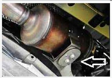
Unbolt the down-pipe support bracket from the down pipe.
